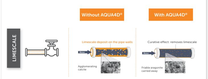
The AQUA4D® technology has an effect on the crystalline structure of the CaCO3 limescale, which changes to a friable, non-agglomerating state, aragonite, and the limescale no longer adheres to the surfaces.
